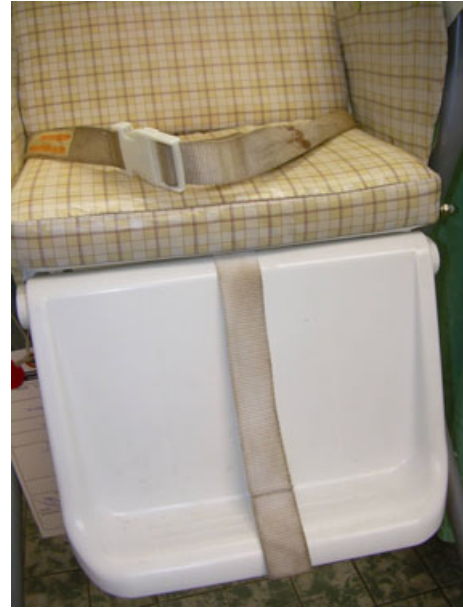
FIG. 3—This was the high chair used by the girl. The leg strap was not buckled to the waist one. The two straps are made up of a very resistant, yet thin synthetic tissue of 3 cm of width. The waist strap is provided with a closing system in "loop clip" and is fixed to both, the left and right sides. The leg strap is fixed at the sat of the seat of the high chair and sticks to a "part guides" on the back of the waist strap closing system. Worth mentioning too, it is a classical high chair with a metal support structure and a seat platform with a removable plastic tray. We also found a certificate of safety at the back of the seat.
